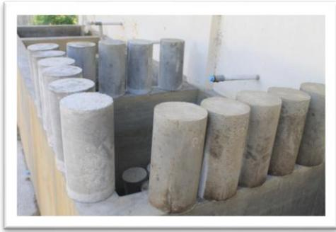
Gambar 2. Benda Uji Silinder Beton
